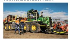
Our Rhino 100 raise borers deliver efficient small-diameter vertical development. These compact machines are fully mechanised, self-contained, electro-hydraulic, mobile, and designed specifically for cost efficient and timely slot raising and backreaming in an underground environment.
