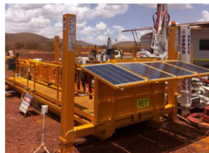
DDH1 Drilling has designed and commissioned a new hands-free, solar powered ancillary sloop for its LF 160 rig operating in the Pilbara.
