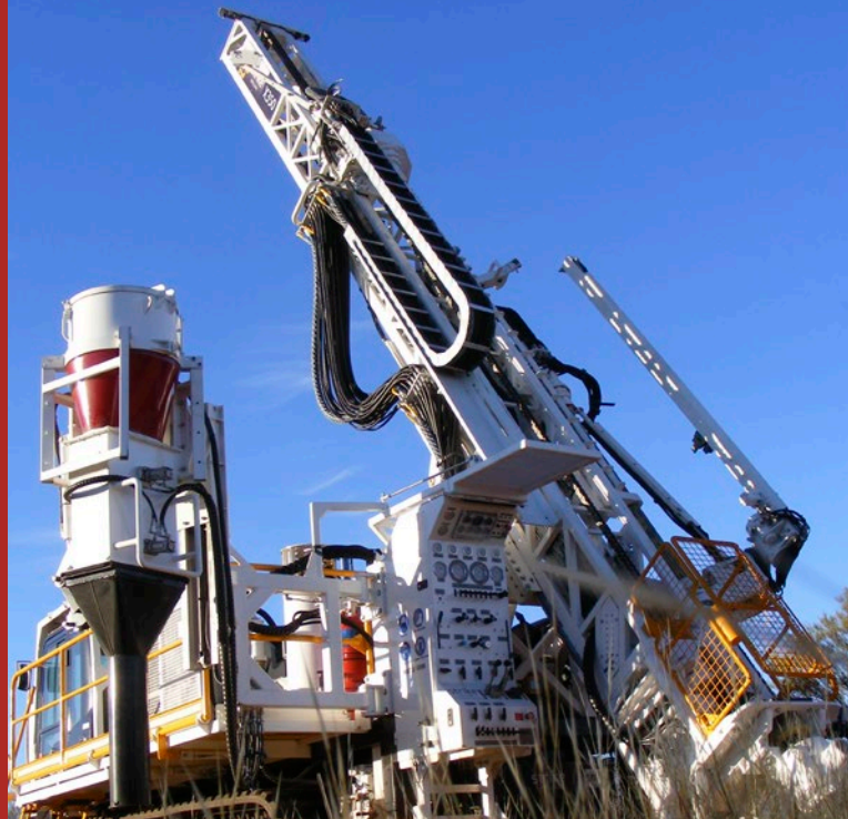
Strike Drilling-Rig 4: Austex X350 dual purpose Aircore/RC Tack mounted rig Midwest WA
